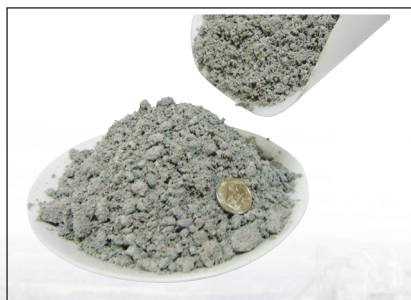
Furnace Bottom Ash
