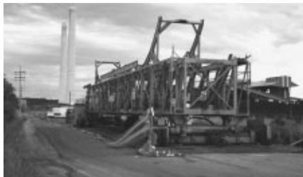
Accelerated Loading Facility (ALF)
