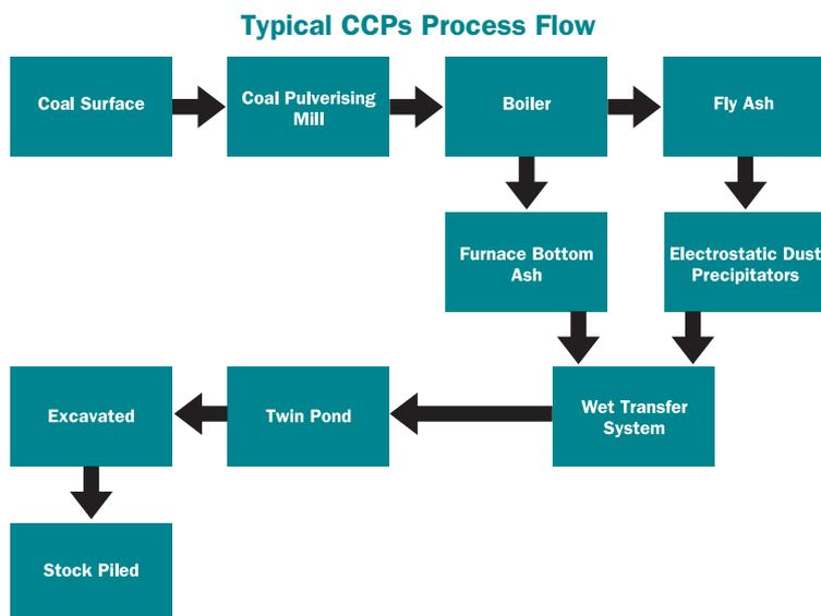
Water used in the wet transfer system, transporting CCPs to storage, is principally sourced from the brown coal mining operations. Brown coal has 60 percent moisture content and is dewatered once removed from the mine site.
