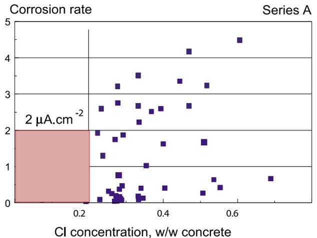
Figure 3: Corrosion rate of steel vs Cl concentration in different concretes and covers
