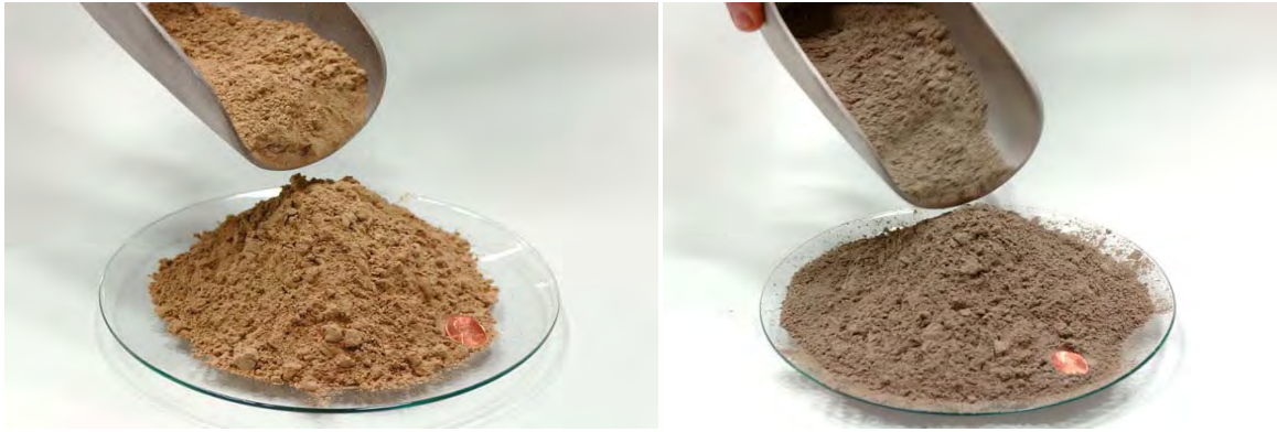
Figure 4 – Fly ash colour variation
