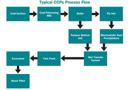
Water used in the wet transfer system, transporting CCPs to storage, is principally sourced from the brown coal mining operations. Brown coal has 60 percent moisture content and is dewatered once removed from the mine site.
