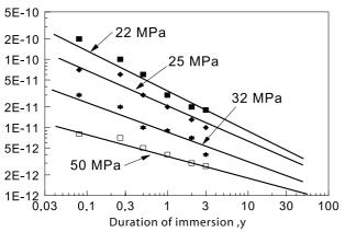
Figure 2: Observed variation of D for concretes of different grades after immersion in seawater.
